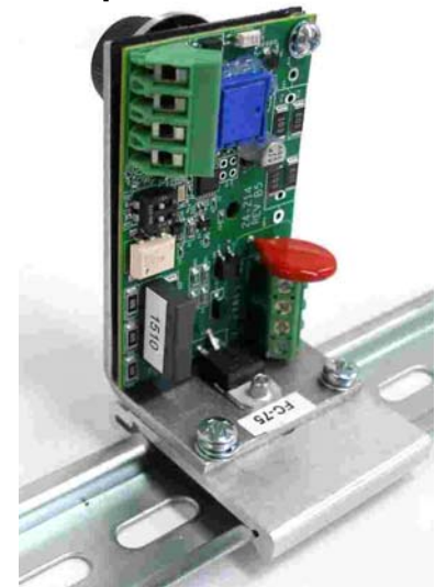
3. Install FC-75 and bracket on DIN rail
